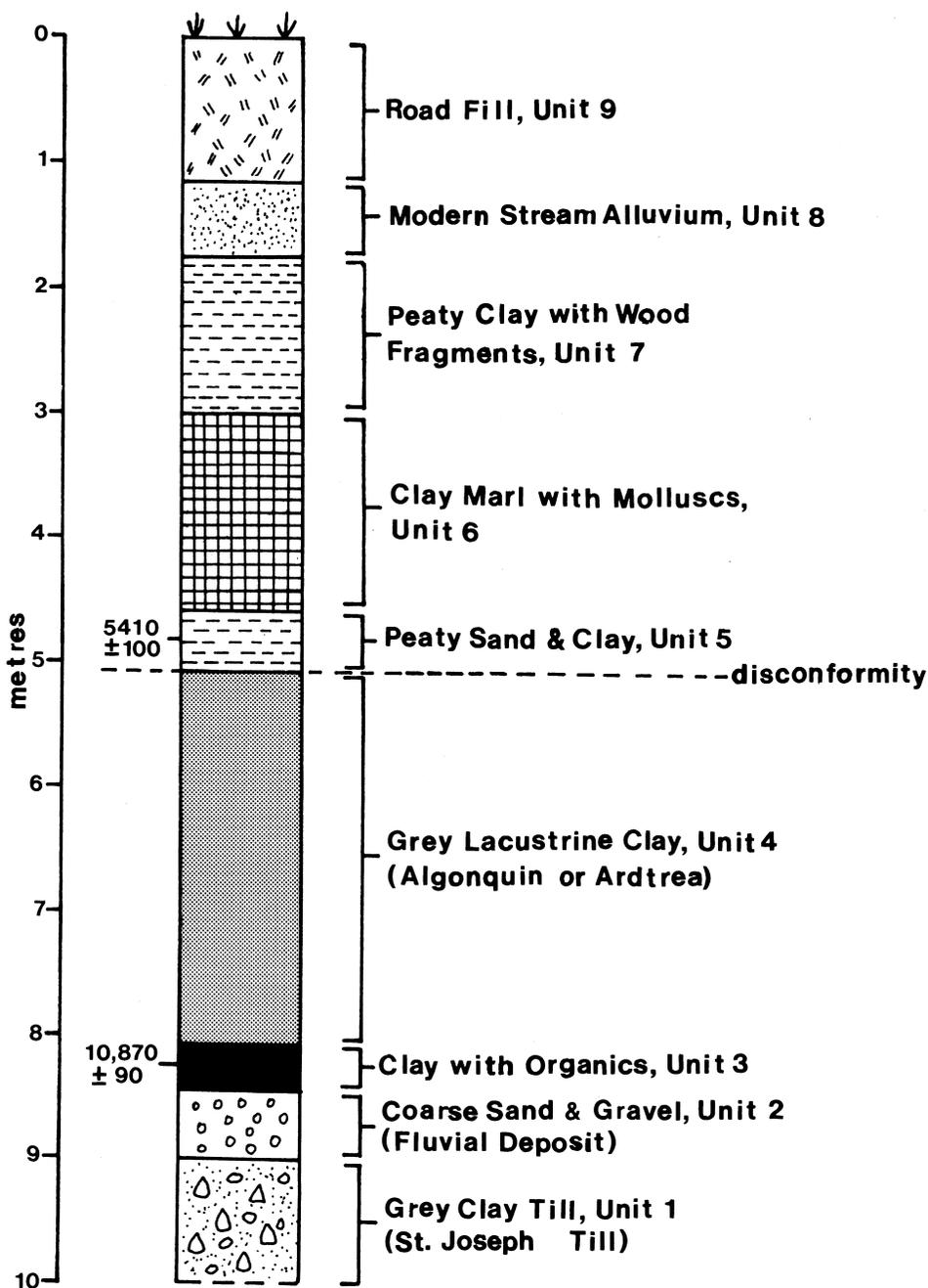
Figure 5. Stylized stratigraphy of Parkhill Creek boreholes.
